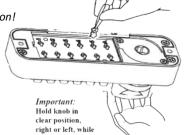
While holding the thumb-turn, remove/add CODE (Red) and NON-CODE (Blue) Tumblers to create your desired code.
